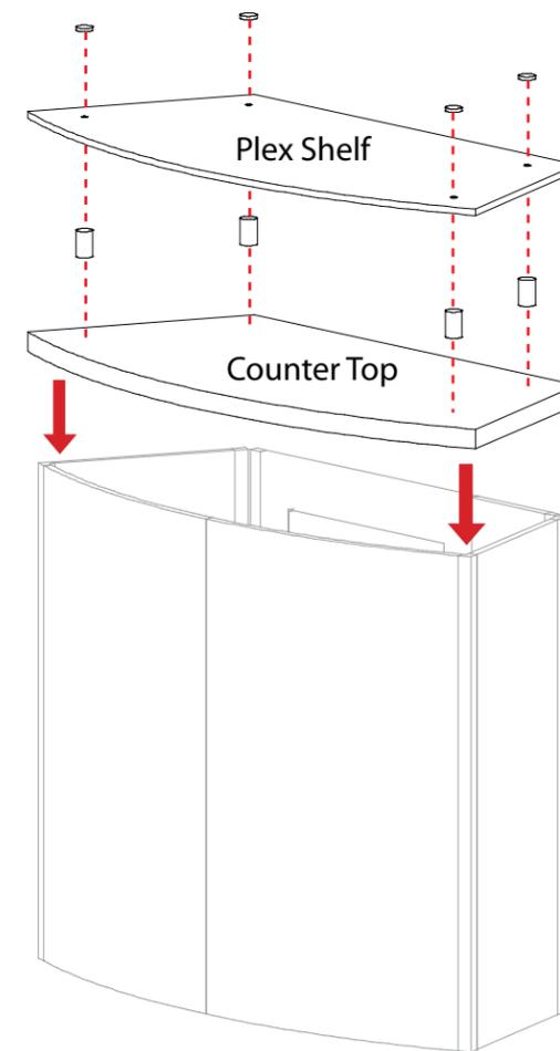
Place counter atop assembled pedestal base. Attach top shelf to counter using stand-offs.
