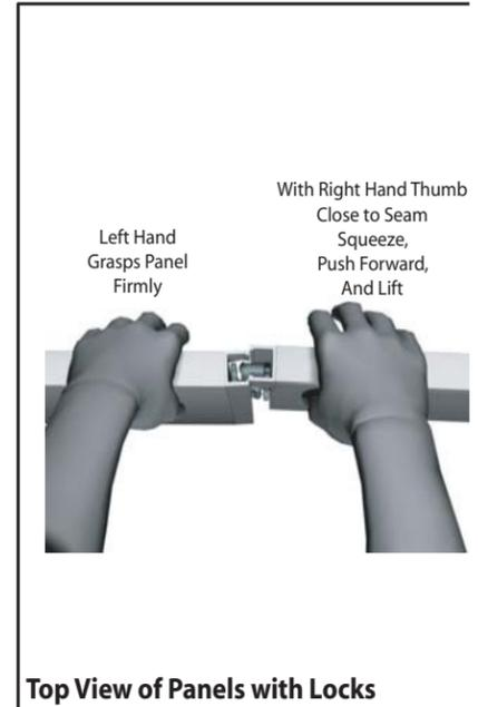
The first level of components contain panel locks that are located at the top of the panel for extra stability and seamless connection. When disassembling panels twist top connection slightly and lift right panel upward.
